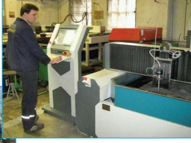
for production needs of the factory, — noticed Mr. Leonid Kontorovich, Technical Director of PJSC "ZTR". — Goods of sheets of different thickness make up 90% of all materials processed by the hydraulic cutting machine. Finished rubber sealings used for different units of the transformer equipment are cut on this machine. Cutting is performed by means of high-pressure water jet in accordance with the program specified by CNC device».
